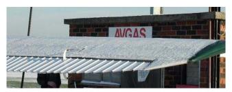
e) Ensure that the entire aircraft is properly de-iced and check visually that **all** snow, ice and even frost, which can produce a severe loss of lift, is cleared. This includes difficultto-see 'T' tails. If water has collected in a spinner or control surface and then frozen, this produces serious out-of-balance forces. There is no such thing as a little ice.
