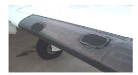
o) Check de-icing boots, particularly the tailplane, for condition, holes etc. Wiping the boots with approved antiicing fluid will enhance their resistance to ice build-up.
