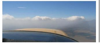
If you fly into the top of clouds, the concentration of water droplets is often greatest near the cloud top and ice could build up quickly.
