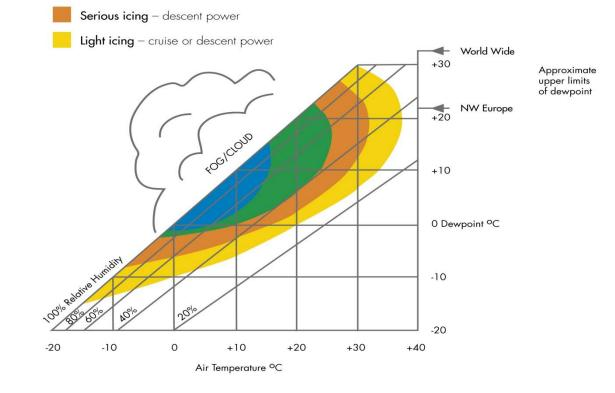
f) Use carb heat as an intermittent ON/OFF control – either full hot or full cold. Do not use carb heat continuously or at high power settings unless the Handbook/Flight Manual allows it. At low power settings, e.g. descent, the application of heat before reducing power, and its continuous use while power is low, is recommended.
