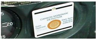
e) 'Spot' type carbon monoxide detectors only have a limited life when unwrapped. Use a 'fresh' one and read the instructions.
