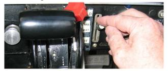
e) Apply full carb heat periodically (every 10-15 minutes) and keep it on long enough to be effective. As a guide, carb heat should be applied for a minimum of 15 seconds, or longer if necessary. The engine may run roughly for a short period while the ice melts.
